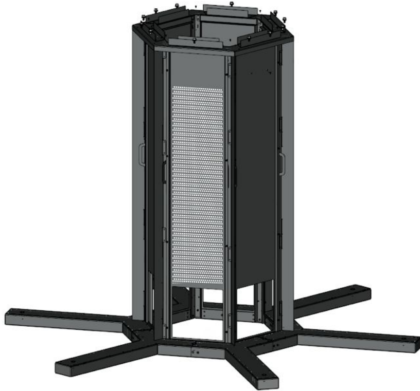
CEC Positioned on Lower Chamber Leveling Base
